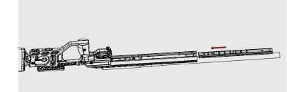
**Step 3:** Align the clearance locations in the Weight with the forend mounting locations in the backbone.
