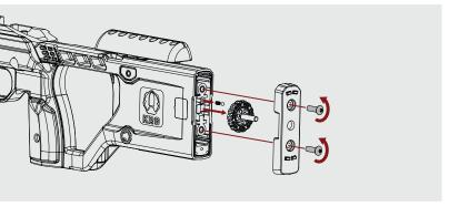
Step 3: Remove pad base from X-Ray stock. Carefully take out the thumbwheel with ball bearing and spring detent inside. You will not need these items for tool-less LOP reassembly, but save these parts if you need to return to the original assembly later.
