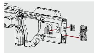
Step 4: Push rear insert mount inside and the LOP lock plugs will come loose. Remove the LOP lock plugs and the rear insert mount. You will not need these items for tool-less LOP reassembly, but save these parts if you need to return to the original assembly later.
