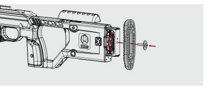
Step 5: Fully thread through and tighten M5X25mm button head screw into M5 flat weld nut. Install buttpad mount plate onto the LOP beam with weld nut/button head screw assembly and tighten in place by turning thumbwheel screw clockwise.
