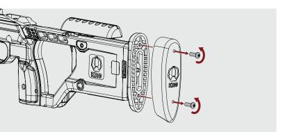
Step 1: Remove the buttpad using a 3mm metric hex/allen wrench. Set aside the buttpad and screws. You will need them for the reassembly (Part 2, step 6).
