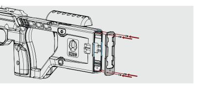
Step 1: Place LOP seal into position and use a light hammer to secure it in place with 4 spring pins.
