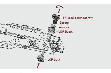
Step 3: Insert LOP bezel on the right or left side of the of the buttstock based on your preference. Insert LOP lock screw on the other side. Install washer, spring and screw on the tri-lobe thumbscrew.
