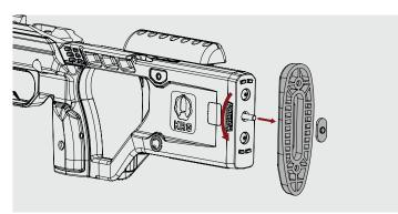
Step 2: Fully unscrew the thumbwheel then remove the weld nut and buttpad mount plate. Set aside the buttpad mount plate and the weld nut. You will need them for the reassembly (Part 2, step 5).
